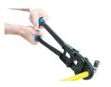
MANUAL TOOL. Position the tool so the press sleeve is completely covered and the tongs are at 90° to the fitting or press sleeve. Close the handles completely so the pressing tongs are completely closed over the press sleeve.
